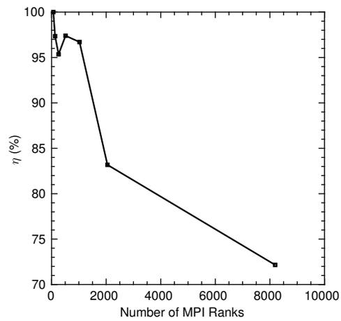
**Figure 5:** Strong Scaling efficiency
